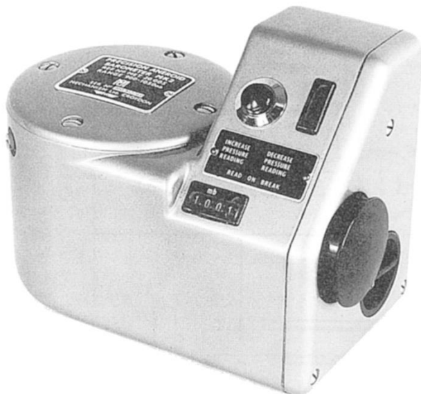
Figure 1. Precision Aneroid Barometer Mk 2—general view, Note the housed static vent on left side beneath cap.
